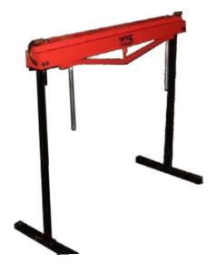
WNS Flange Folder is designed to create a right angle flange on pre-cut sheet material. This machine provides quick easy folding of material up to 1mm (20 g) as there is no need for clamping. It is also ideal for use with Pittsburgh lock rollformers. Another advantage of this machine is that it is open-ended.
