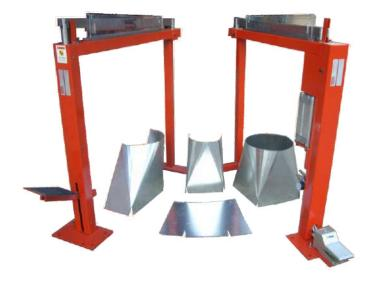
It can form 1.0mm thick metal up to 450mm long & 0.8mm up to 600mm long giving accurate & consistent forms. The pre-cut blank is located on a pivot at one end, which allows the blank to turn.
